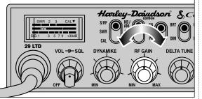
• Rotate the O RF Gain knob counterclockwise to reduce gain in strong signal areas. In weak signal areas turn clockwise to increase gain.
